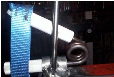
NOTE: the end of the gripper is showing slightly out of the tube, when positioned correctly the end of the gripper should not protrude. The small amount of protrusion should not affect the results of the measurement but we tried to be very consistent with gripper positioning.
