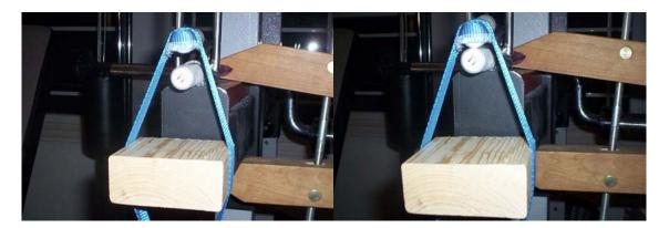
Here a GM is loaded and a block of wood is used as a spreader. The goal is to not allow the strap to contact the fixed leg of the gripper and throw off the calibration. The picture on the left shows the loading pin loaded with 125 pounds. The picture on the right is when the gripper just closed with 150 pounds on it. In the picture the gripper looks close to the metal rod on the left, but it is not touching it.
